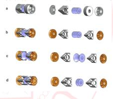
gives a much higher, but less homogeneous microwave field for short samples or paramagnetic states produced by laser excitation. The sapphire ring is depicted in pale blue, the Teflon supports in white and the metal end pieces in silver or copper.
